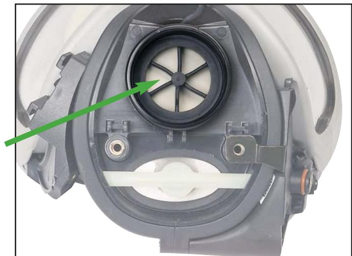
*The Inhalation check-valve allows air to flow only in one direction when a facepiece is pressurized, helping to protect a shared-use regulator from contamination.*
